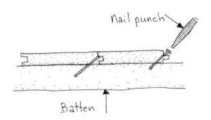
When cutting boards, always cut them face up to prevent marking of the exposed surface. Last board will most likely require trimming to width by cutting and planing the tongue edge.
